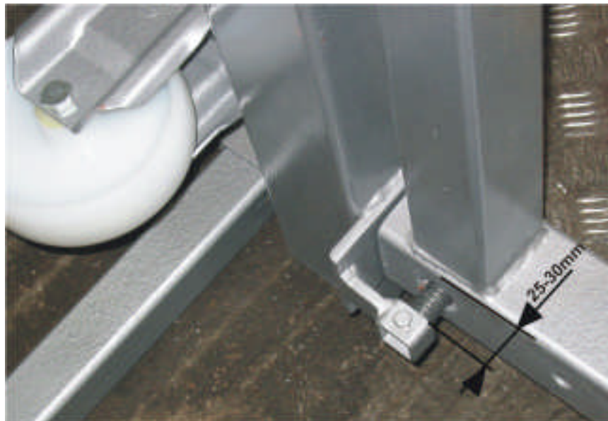
Fig.8 The swingarm spring shall be tensioned to proximity 25-30mm out from its position of rest with help of the flux support out/in slide.
