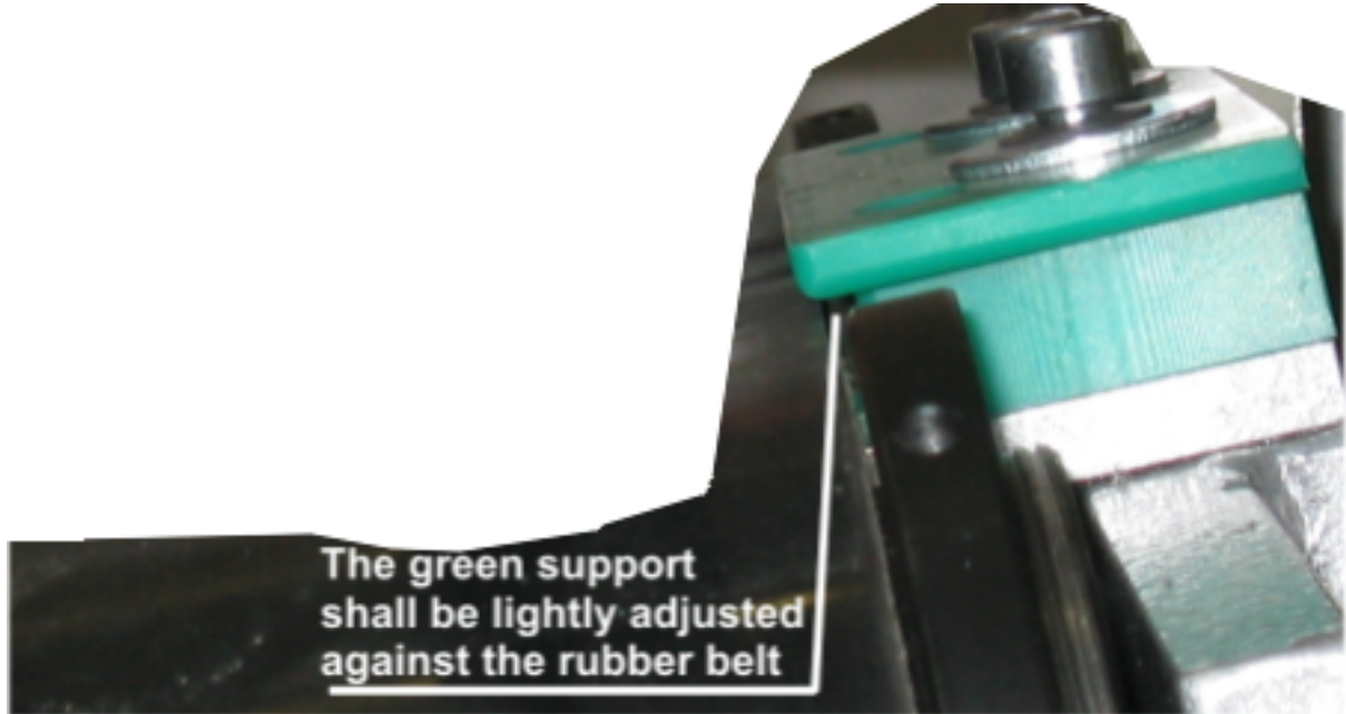
Fig.4 The green belt support shall be lightly adjusted against the rubber belt.
