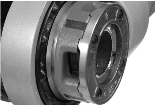
Figure 15 – Pipe Even with Edge of Dies
