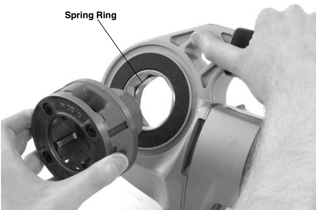
Figure 9 – Installing Die Heads into 600-I Power Drive
