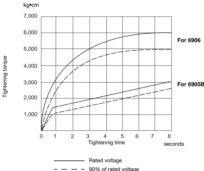
Hold the tool firmly and place the socket over the bolt or nut. Turn the tool on and tighten for the proper tightening time.
