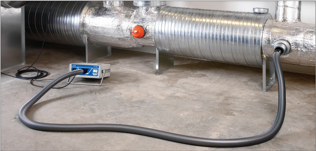
Figure 3: Connection to the duct system
