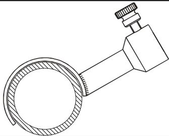
A technical drawing of a shell-shaped wire spiral guide. It consists of a circular ring with a spiral wire wound around it. The ring is attached to a rectangular block with a threaded hole on top. | <p>Führungsbügel zur Führung der Drahtspirale in Schalenform</p> |
