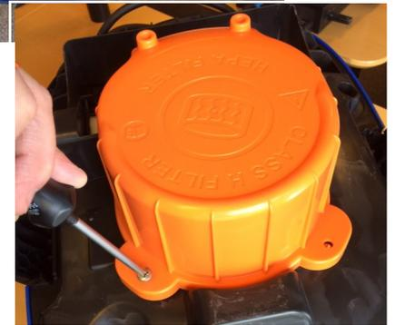
Open the container clamps (fig.1) and turn motor head upside down. Unscrew and remove the orange filter cover (fig.2).
