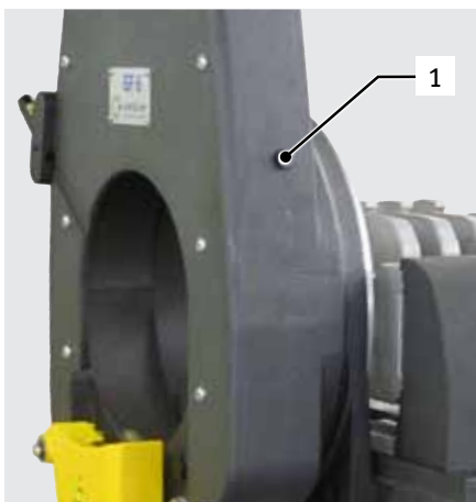
Position of the safety screw for the GF 4 and GF 6 (AVM/MVM).
