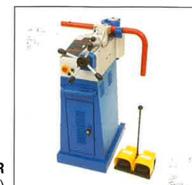
SUPER BENDER \varnothing 64 x 2 mm. (max)
