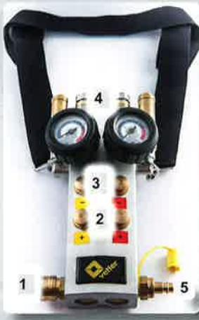
Connect the connection hose from the pressure reducer or the air-supply hose to the inlet coupling (1) of the control element. To secure the brass eyelet of the coupling, twist against the lock pin. Connect the adapter nipple of the filling hose to the outlet couplings (4) of the control element. Comply with the side identification of the coloured filling hoses. Check to make sure the filling hoses (safety couplings and nipples) have latched.
