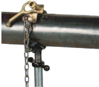
1. Insert chain end of hold down device through containment loop and tighten set screw to half the length of chain
