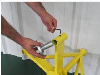
Caster stem inserts into base socket and must be secured with the provided Allen screw and wrench
