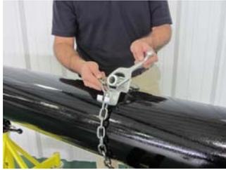
4. Make sure Hold down device chain is tightly secures load to vee.
