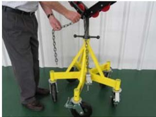
2. Back off adjustment screw in order to have maximum thread travel
