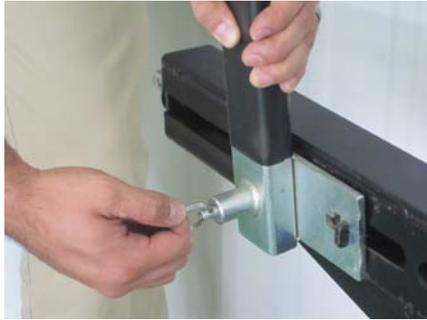
To clamp narrow width loads, clamp fork should be with plunger pin nearest to the center of the head.
