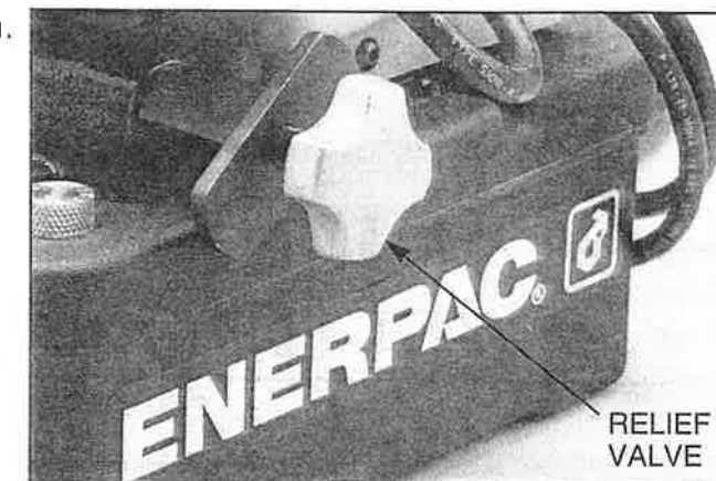
Figure 1 - Pump Relief Valve
