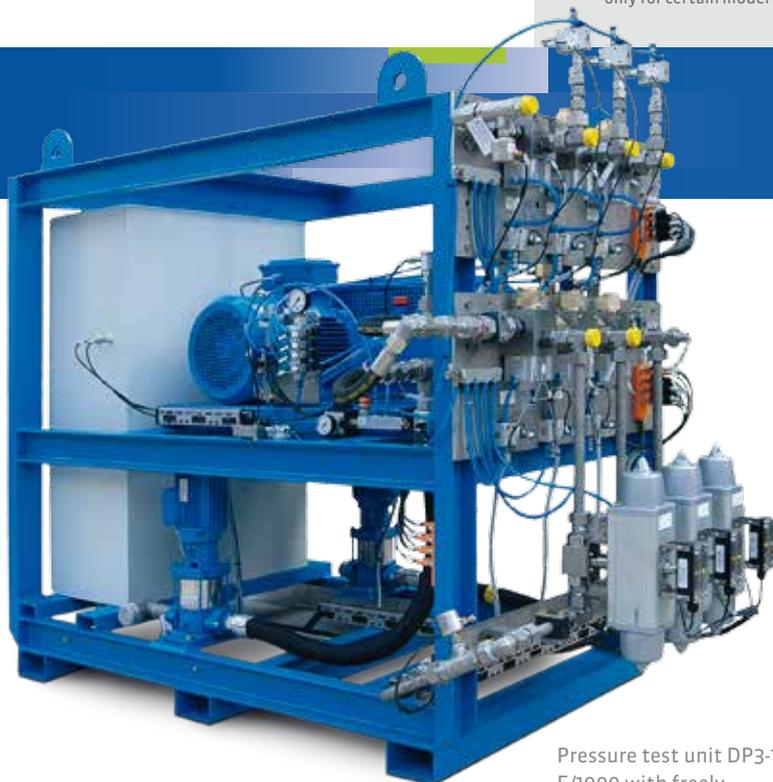
Pressure test unit DP3-10 E/1000 with freely programmable pressure curve
