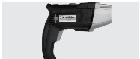
Electric variant (RPG 3.0): Set the switch in the center position to block the On/Off switch
