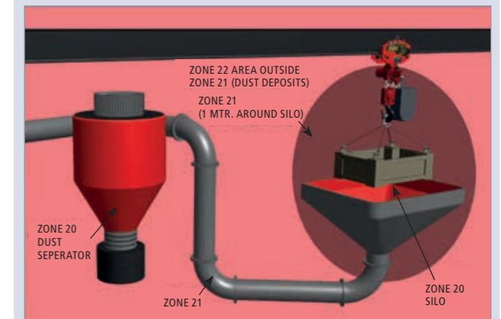
The above diagrams are simple examples of explosive atmospheres within industry. Each site may differ.
