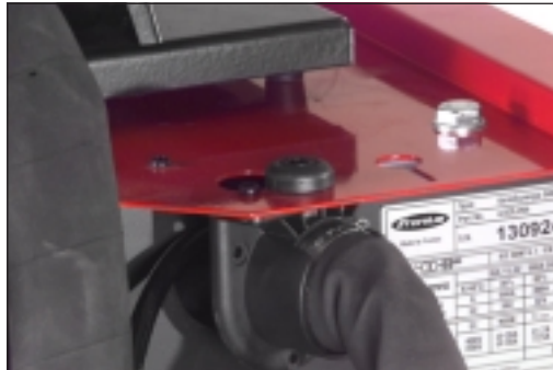
Fig.21 Fitting the interconnecting hosepack to the power source
