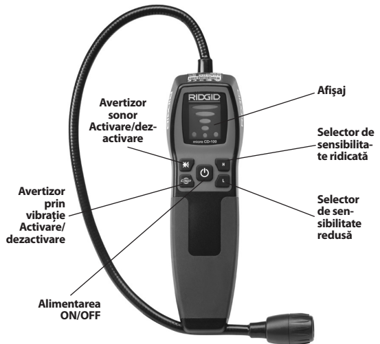
Figura 2 – Componentele micro CD-100
