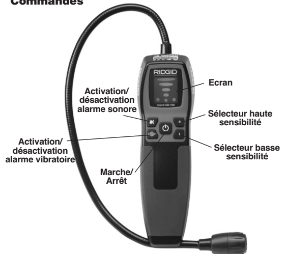
Figure 2 – Composants du micro CD-100
